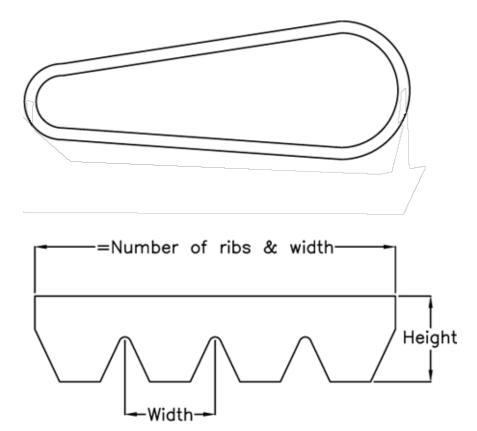
$\begin{aligned} \text{Datum Llength} &= 1244 \\ \text{Height} &= 3.5 \\ \text{Number of ribs} &= 9 \\ \text{Pitch} &= 2.34 \end{aligned}$
